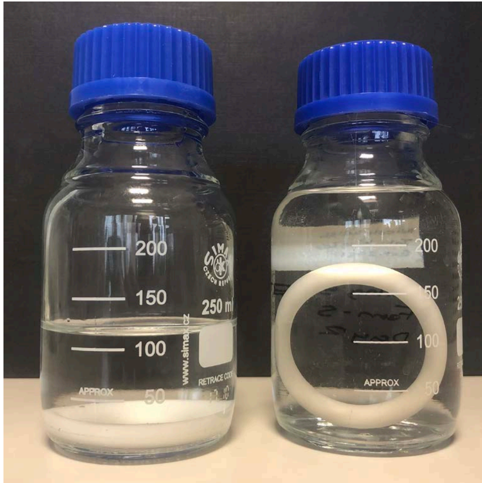
Fig. 3. Sealed glass flasks for in vitro release testing of drug-releasing vaginal rings. A – ring allowed to rest on bottom of flask containing 100 mL of release medium. B – ring suspended by a nylon thread in glass flask containing 200 mL release medium. The nylon string can be seen in the space between the release medium and the blue screw-top lid.
