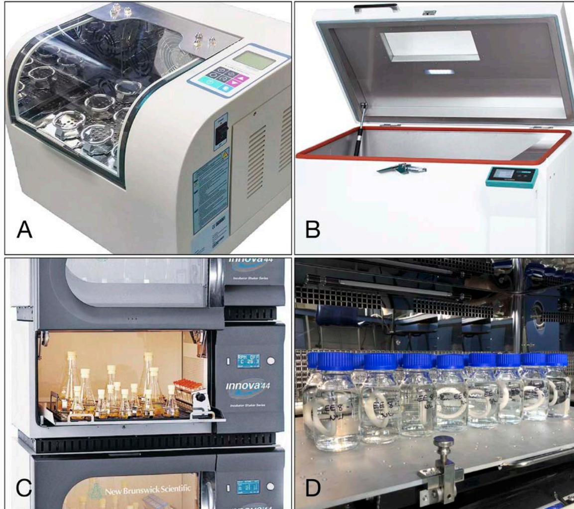
Fig. 2. Different type of shaking incubators commonly used for in vitro release testing of vaginal rings. A – a benchtop shaking incubator; B – a floor-standing top-opening orbital shaking incubator; C – stackable orbital shaking incubators; D – flasks containing suspended rings, and stored in an orbital shaking incubator.
