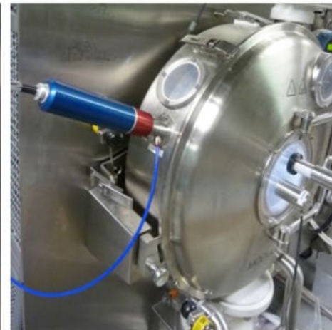
Coater Closed with PhAT probe in place looking into cascade
