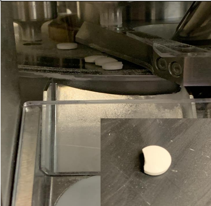
Lactose Blend + 10% vardenafil: Breakage at 7-10 kN
