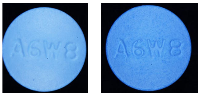
Figure 7. Comparison of Calcium Carbonate (left) and Calcium Carbonate with Isomalt (right) at 2% Theoretical Weight Gain
