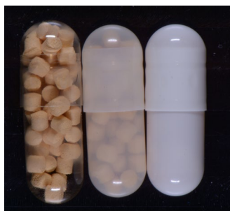
Figure 10. Hypromellose Capsules, No Opacifier (left) Calcium Carbonate (middle), E171 (right)
